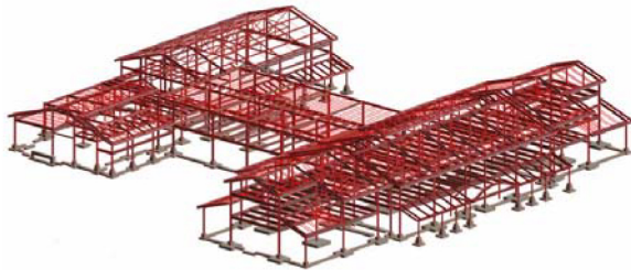
A Revit Structural Model designed by JBA.
